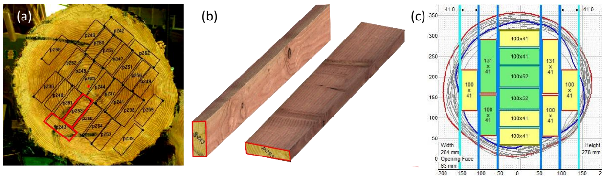
Figure 1: (a) Log end image in a sawmill from TreeTrace project with board ends drawn on it (boards N°243 and 253 highlighted in red colour); (b) isometric view of optical scanning of the two aforementioned neighbour boards; (c) example of a software optimizing the sawing pattern of a log (Saatech systems 2021).
